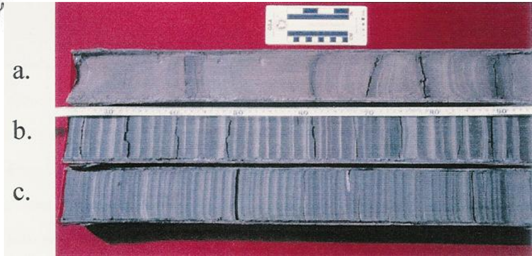
Photograph of cross-section cores from UMass Amherst NGES at (a) 32 m, (b) 7.6 m, and (c) 3 m depth.
