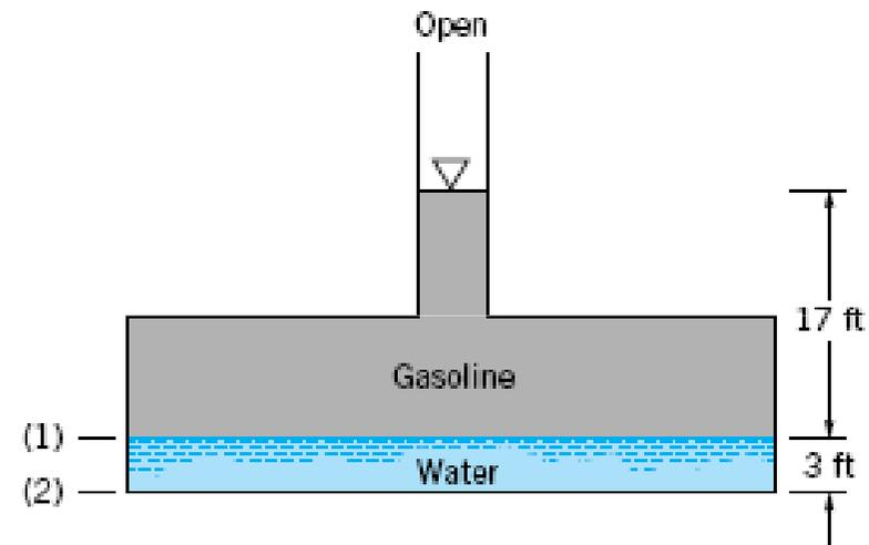
$$\rightarrow \frac{p_2}{\gamma_{\text{H}_2\text{O}}} = \frac{908 \text{ lb/ft}^2}{62.4 \text{ lb/ft}^3} = 14.6 \text{ ft}$$
