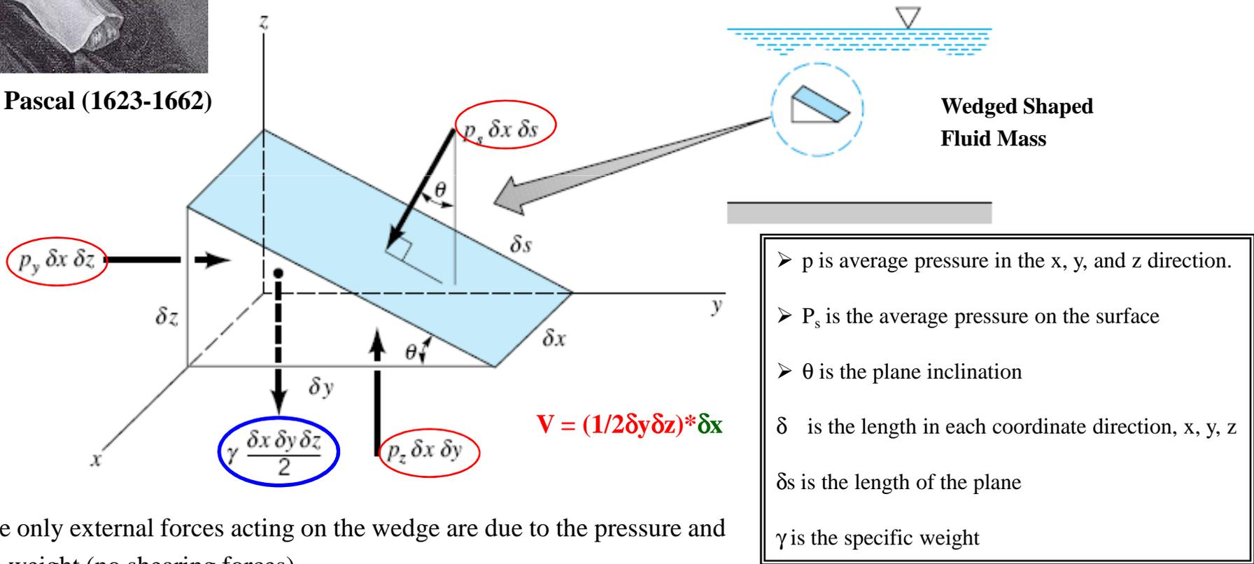
➤ The only external forces acting on the wedge are due to the pressure and the weight (no shearing forces)
