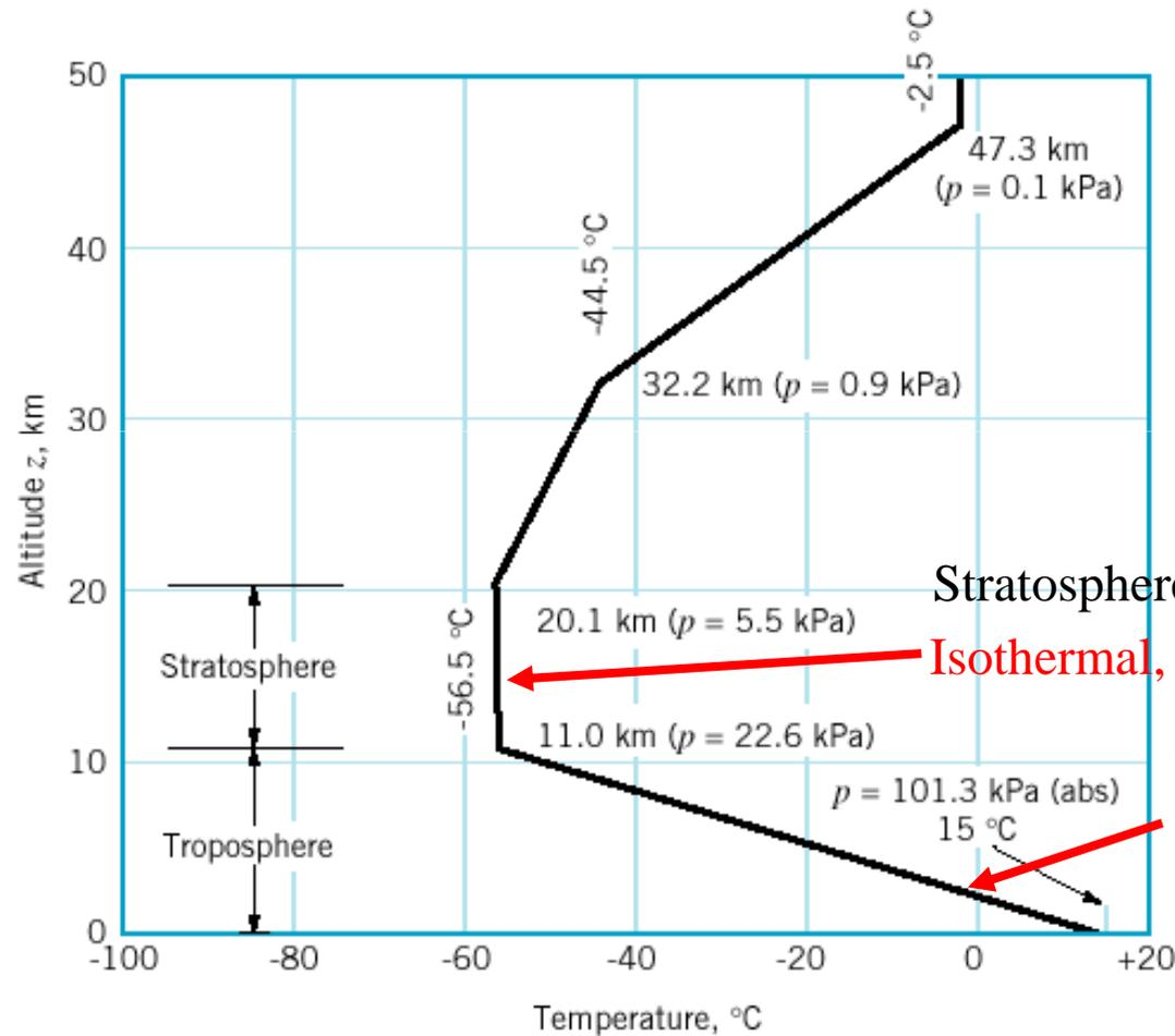
Standard Atmosphere is used in the design of aircraft, missiles and spacecraft.
