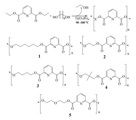
To force the reactions to completion titanium tetraisoproposide  $[Ti(O-iPr)_4]$  was added as Lewis acid catalyst, and reaction temperatures were raised to 180 °C to promote elimination of ethanol. Scheme 1 shows the condensation reactions and the prepared polymers.
